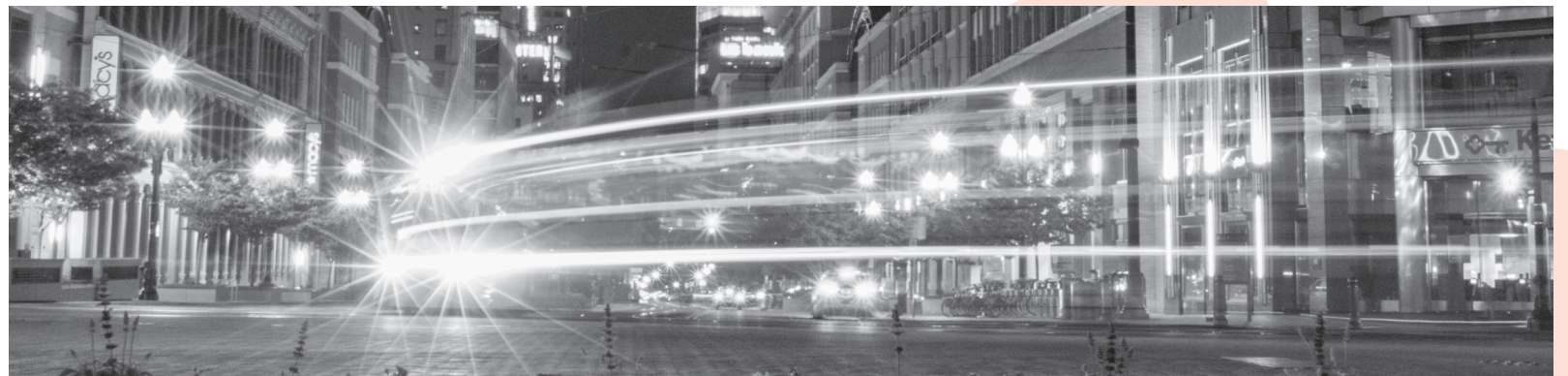
The streetlights of downtown Salt Lake City have old-time character but spill light in all directions and up into the sky. With no shielding, the exposed globes cause glare, making it difficult to see and disrupting wildlife.
