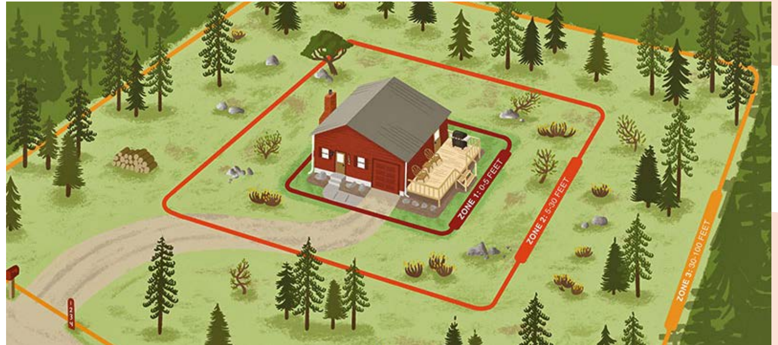
Defensible space can reduce the spread of wildfire to homes, buildings, and mature trees. Courtesy Colorado Forest Service.
